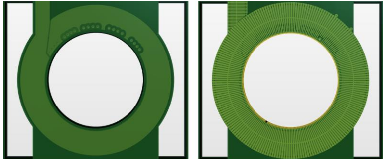
Fig. 1. PCB inductors: original inductor (left), shielded-windings inductor (right)
